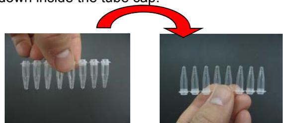
2. Place the reaction tubes cap-side down on the lab bench for 2 minutes. This allows the solution to reconstitute the dried LAMP reagents inside the tube caps. Make sure no fluid is stuck at the end of the reaction tube.
