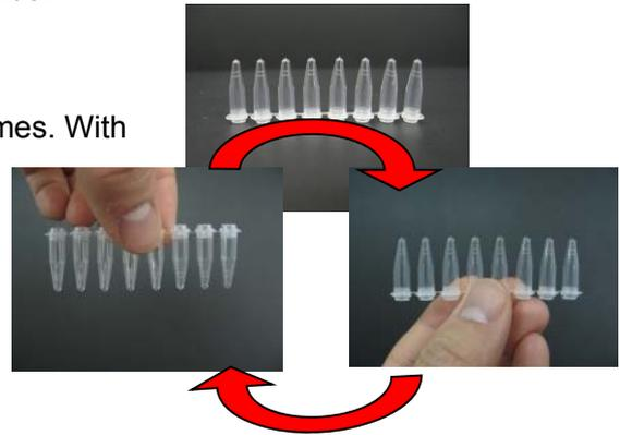
4. Finally, shake the reaction tubes downward to collect the solution at the bottom of the tubes.
