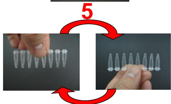
bottoms to the caps. This ensures proper mixing and dissolving of the LAMP reagent.
