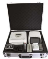
Figure 1: A Truelab Real-Time PCR workstation field case
